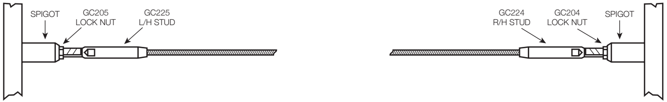
System 5: Swage stud with left & right hand M8 thread and welded spigots
