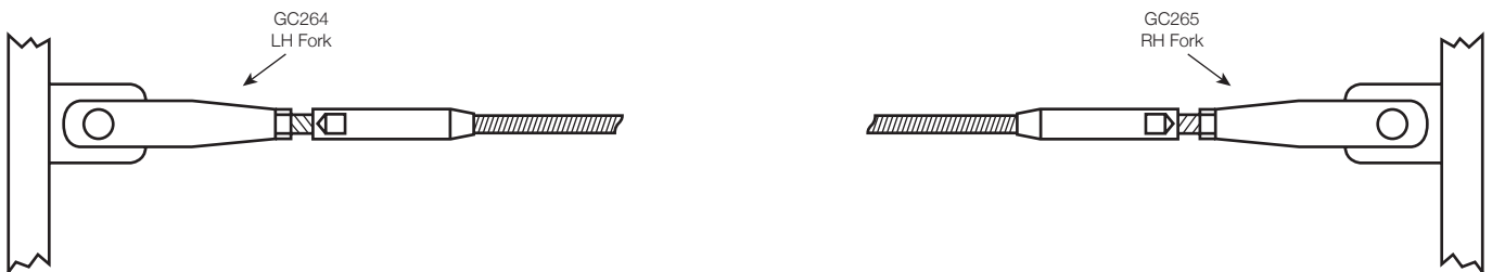
System 9: Swage stud with metric thread both ends
